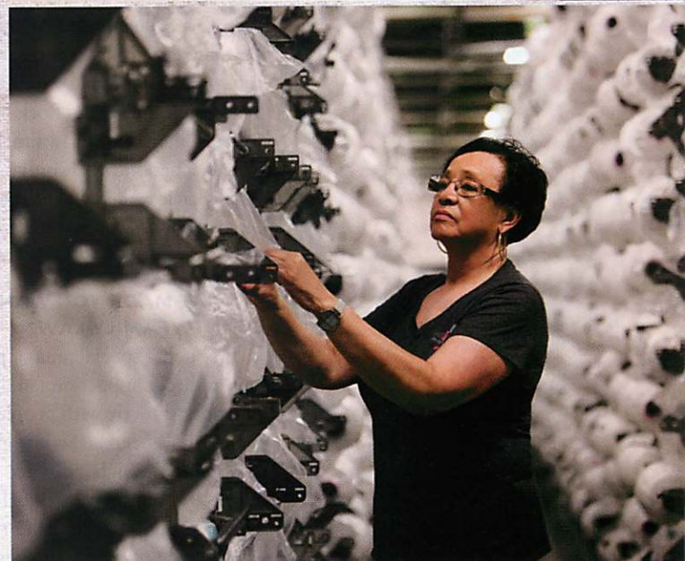
▲ Fairystone Fabrics operates 24 hours a day, 365 days a year. Idling machines causes cooling that leads to more equipment breakdowns, owner Jim Bryan says.
